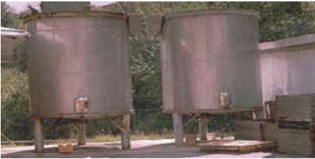
Water tank for curing chestnut
