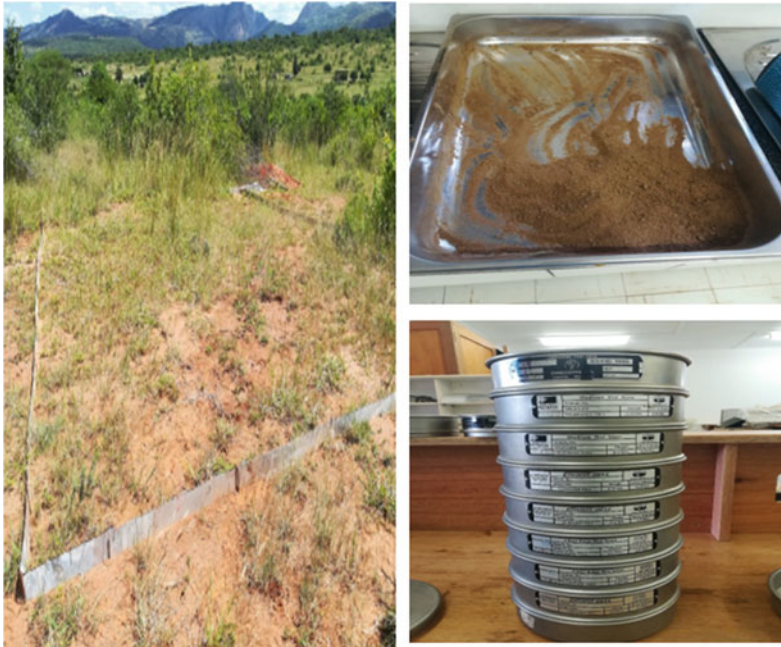
Fig. 3.5 Runoff plots, sediments, and particles sieves used during experiments
