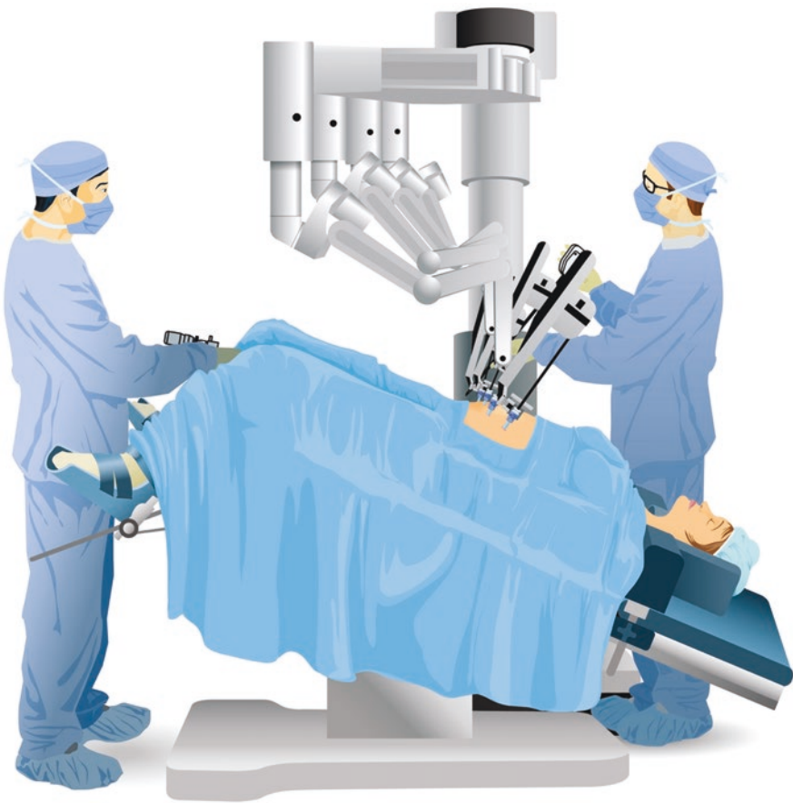
Fig. 11.3 Schematic drawing depicts patient placed in steep Trendelenburg position and Docking of the Xi ® Da Vinci Surgical System on the side of the patient
