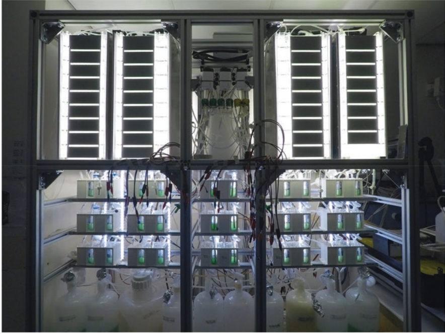
Fig. 1 Fully inoculated Living Architecture “wall” and apparatus installed at the University of the West of England, Bristol. (Photograph courtesy of the Living Architecture project (2019))
