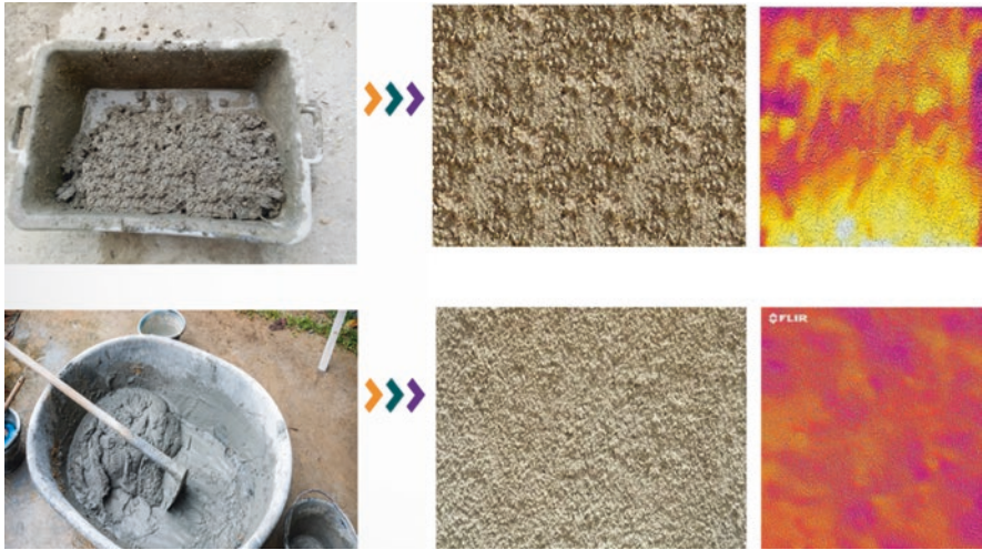
Fig. 8 Rough texture with different concentration of palm particles aggregate. (Source: Adapted by Boukhelkhal Islam, 2020)
