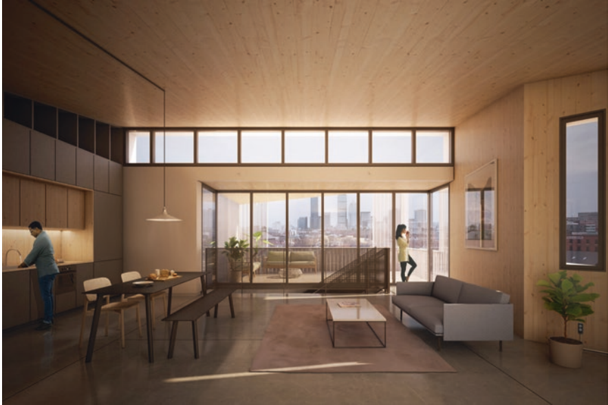
Fig. 19 Locally sourced and trimmed CLT will be exposed in indoor spaces. (Credit: Generate | Placetaylor)
