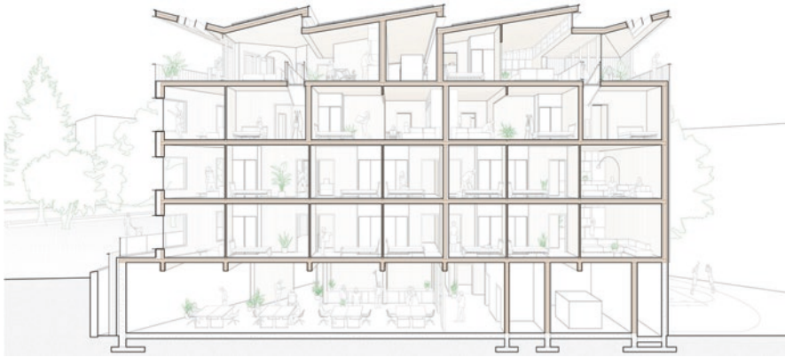
Fig. 15 The building section displays the array of interior spaces including the 14 residential units and co-working space. Credit: Generate | Placetaylor
