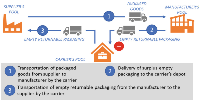
Fig. 8. One typical cycle of Switch-pool, if the quantity available at the manufacturer exceeds the quantity of empty packaging to be returned and the carrier delivers the full quantity
