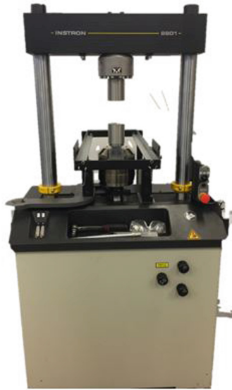
Fig. 2. Instron 8801 prepared for the compression test [author]
