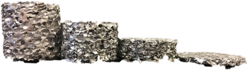
Fig. 7. The steps of the free compression of the foam (0–30–50–80% strain) [author]
