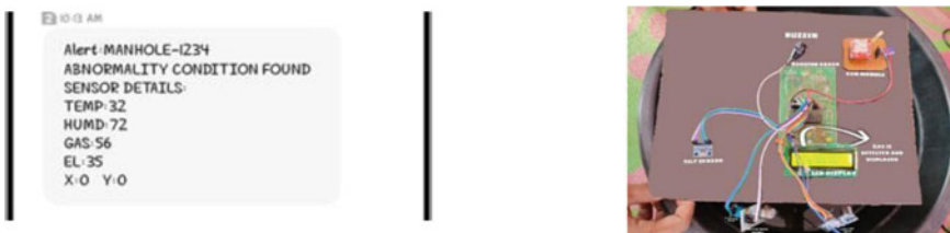
Fig. 8 Manhole detection using a gas sensor
