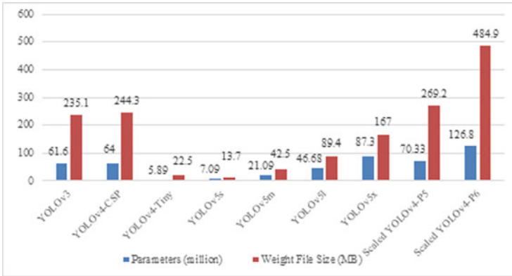
Fig. 3 Comparison of various YOLO models based on parameters and weight file size
