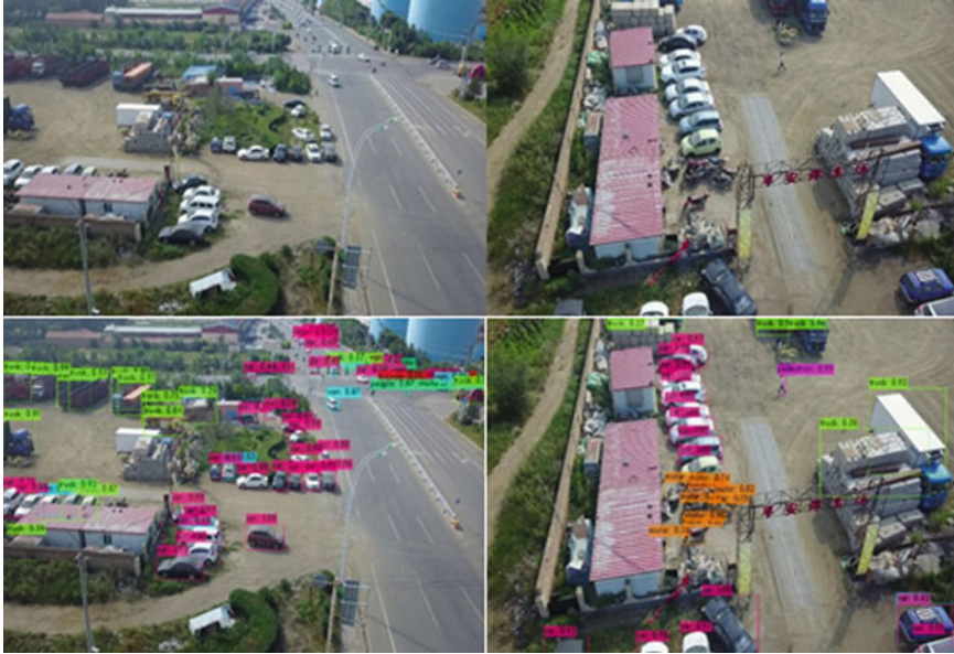
Fig. 7 Visual results of object detection on test-set images of VisDrone (above) Actual image from test set (below) Output image with bounding boxes and confidence score for the detected objects
