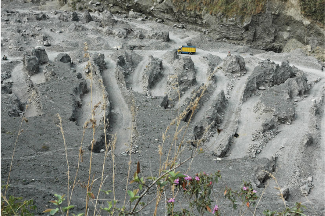
Fig. 3.8 Example of block and sand mining of Merapi volcanic deposits taken at Kali Gendol and showing the mining of block-and-ash flow deposits from the 2006 eruption. Photo credit Sylvain Charbonnier
