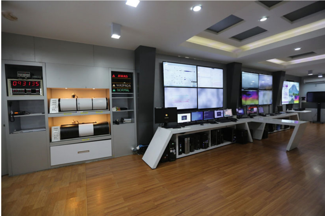
Fig. 13.5 The Merapi monitoring room at BPPTKG office (photograph taken in 2020). The telemetry data, such as seismic, deformation, gas, and visual data from
