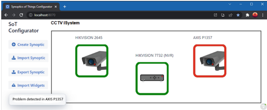
Fig. 4. Synoptic for the CCTV system
