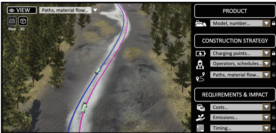
Fig. 4. Application interface. On the left, is an example of a 3D view of vehicle paths. On the right, are possible factors to manipulate and simulate in the virtual environment.
