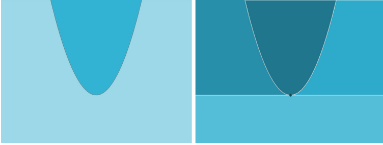
Fig. 1. CADs sign-invariant for x^2 - y in the two possible orderings. The ordering y \succ x generates the CAD on the left with only three cells (the coloured regions and the curve between). The ordering x \succ y generates the CAD on the right with nine cells (the four coloured regions along with four line segments and the turning point of the curve).
