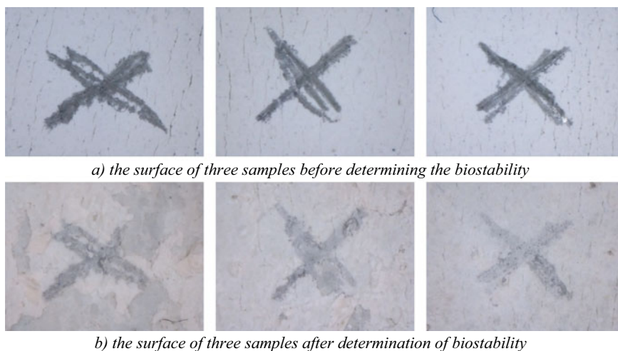
Fig. 10 Photos of the surface of paintwork samples filled with activated kaolin before a and after b determination of their biostability
