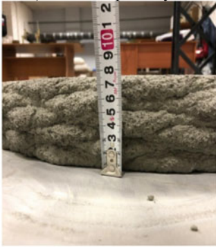
c) deviation of the height of the product layers from the design value
