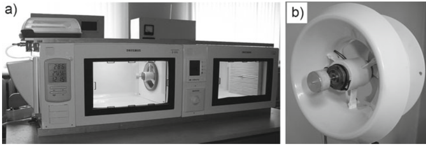
Fig. 1 External view of a monoblock air supply unit with a humidification module a and a spraying unit with the PRA b
