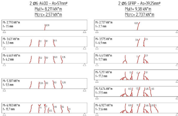
Fig. 16 Typical stages of crack development in beams reinforced with two bars 2 Ø6 A400 and 2 Ø6 GFRP
