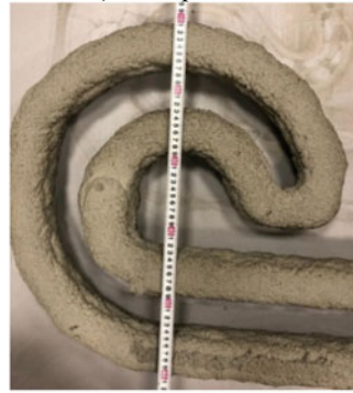
d) deviation of the product length and width from the design value, the influx in the starting point
