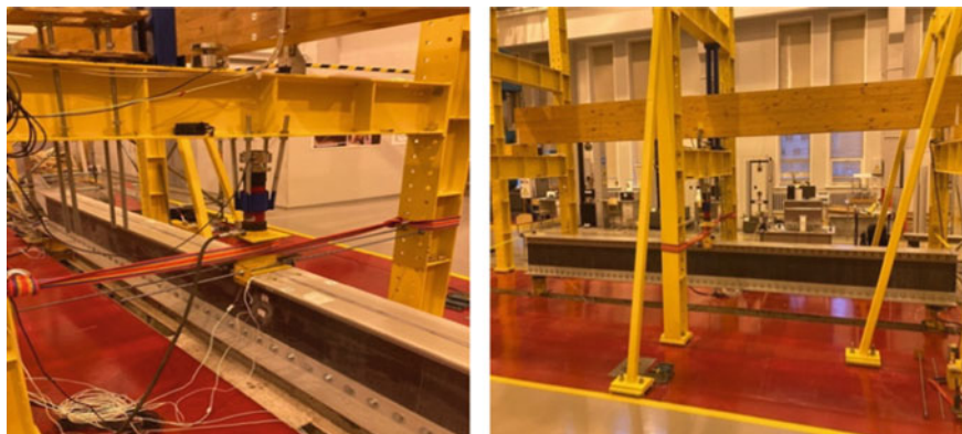
Fig. 2 The composite I-beam with a solid web of PFP before full-scale test
