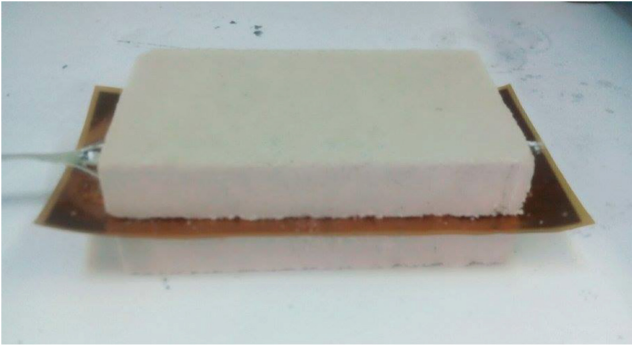
Fig. 3. THB sensor inserted between two green sand samples
