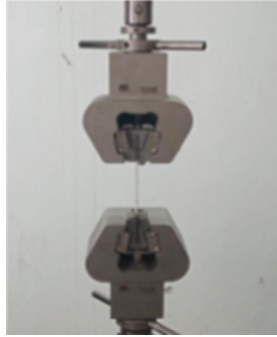
Fig. 2. Tensile test set-up
