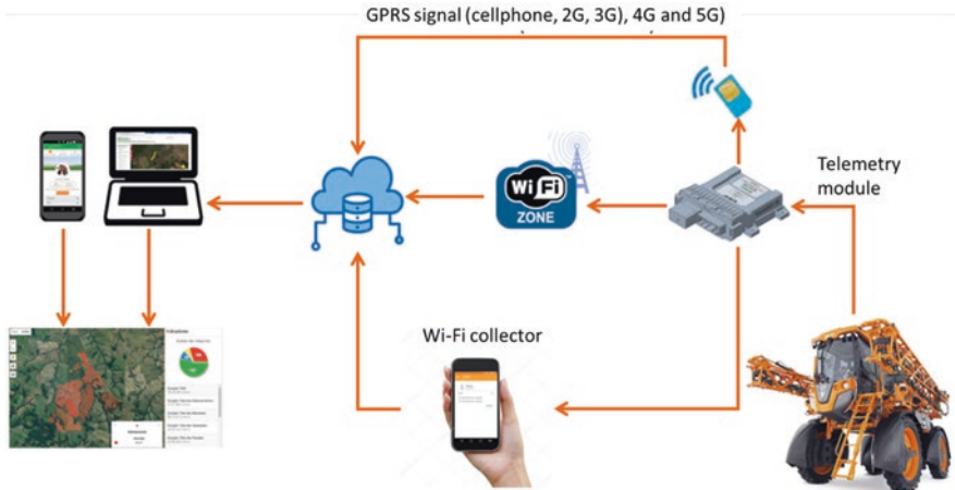
Fig. 13.5 Example of a telemetry system of a self-propelled sprayer. (Source: Adapted from Jacto 2019)
