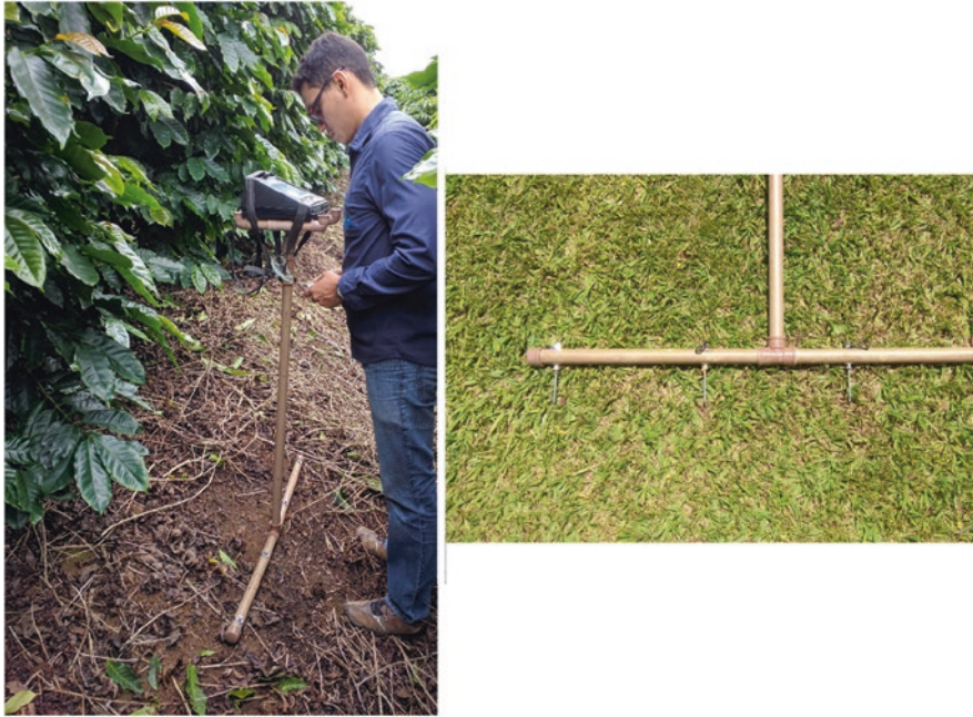
Fig. 8.6 Portable soil apparent electrical conductivity sensor. (Source: Queiroz et al. 2020)
