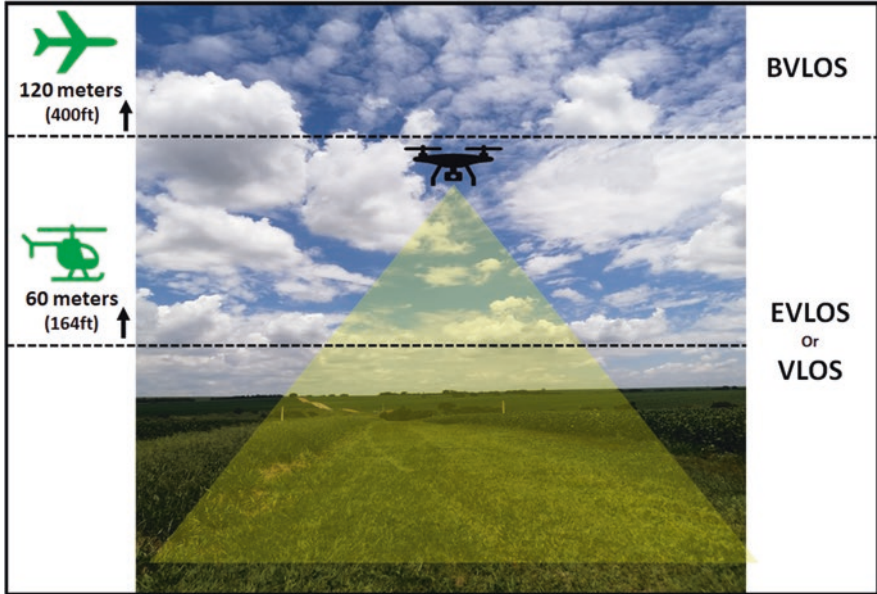
Fig. 7.1 Air traffic zones by operation altitude and respective visual categories. BVLOS beyond visual line of sight, EVLOS extended visual line of sight, VLOS visual line of sight
