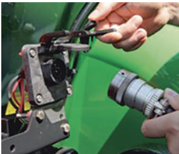
Fig. 15.1 ISOBUS: Standardized communication protocol between different agricultural machines. (Source: AgLeader 2020)
