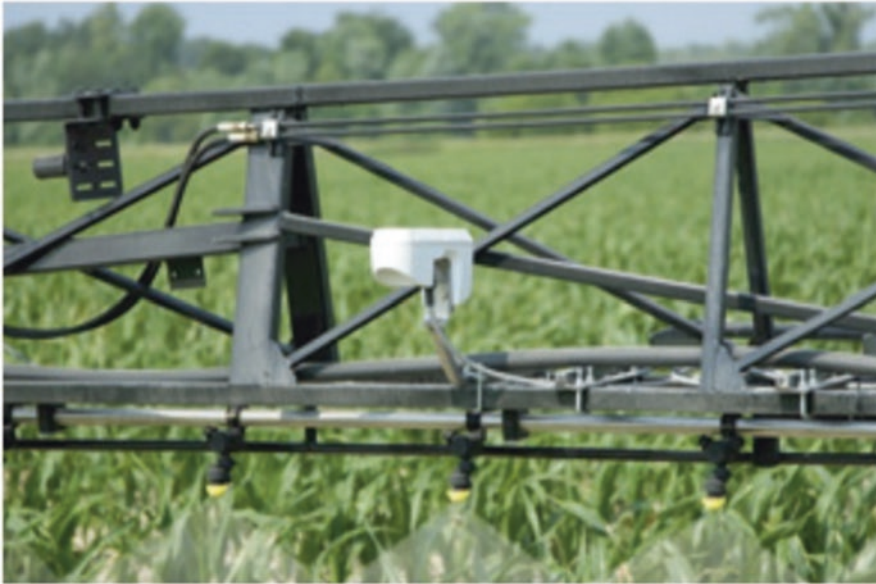
Fig. 8.8 GreenSeeker sensor for variable-rate application of nitrogen. (Source: Trimble Navigation Limited 2013)
