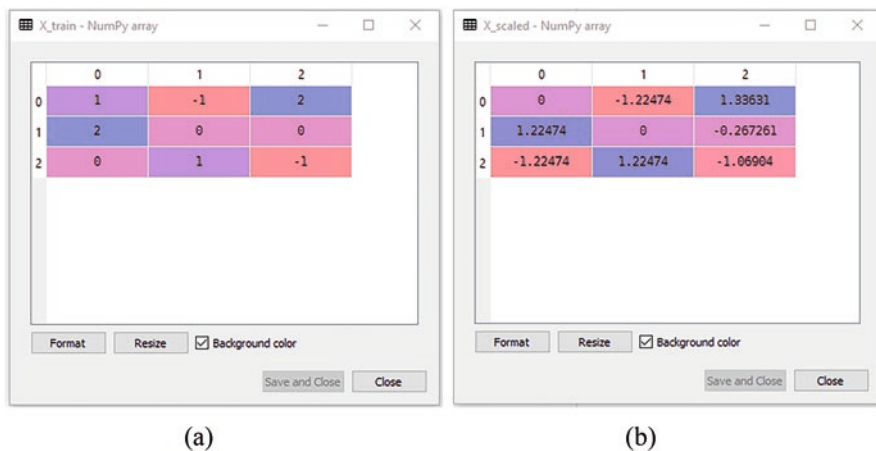
Fig. 14.2 (a) Result stored in the X_{train} variable, (b) result of the transformation of the X_{train} variable stored in the X_{scaled} variable. (Source: Authors)
