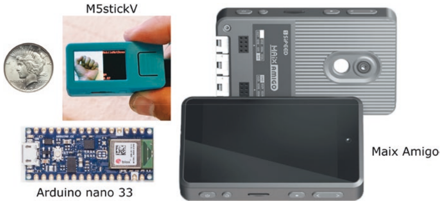
Fig. 12.8 Arduino Nano 33 IoT and two embedded systems based on K210 MCU: m5stickV and Maix Amigo
