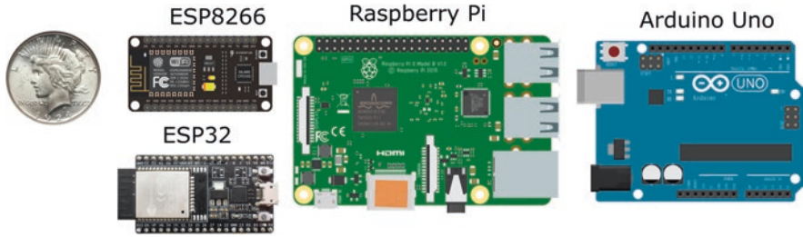
Fig. 12.7 Four popular embedded system boards: Arduino Uno, ESP8266 (or NodeMCU), ESP32, and Raspberry Pi3 B (The coin diameter is 30.6 mm)
