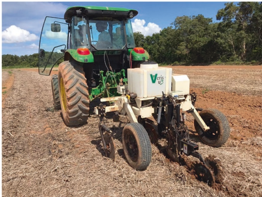
Fig. 8.5 Veris Technology's U3 platform, which integrates sensors of soil apparent electrical conductivity, pH, and reflectance. (Source: Authors of this chapter)
