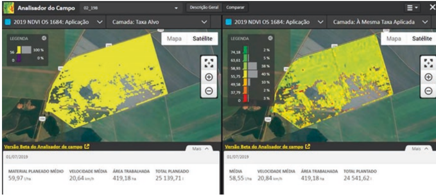
Fig. 17.7 On the left, the map planned for the application, and on the right, the map that was executed by the machine. Costa Rica, MS. (Source: SLC Agrícola)
