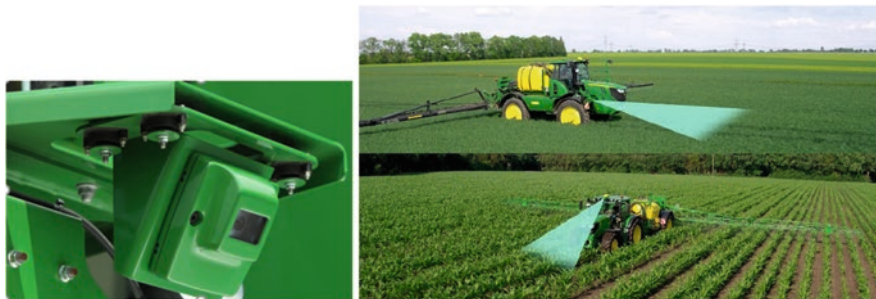
Fig. 9.5 John Deere's AutoTrac Vision System. (Source: John Deere)
