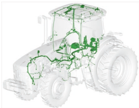
Fig. 13.3 CAN bus from an agricultural tractor. (Source: John Deere 2018)
