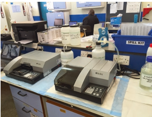
Fig. 3.2 Major equipment required for manual ELISA; a microtiter plate reader for quantifying colorimetric signal intensity (left) and a microtiter plate washer (right)
