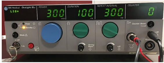
Fig. 10.8 A diode laser (Iridex, CA). Normal laser settings for laser coagulation of a ROP newborn
