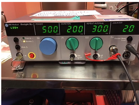
Fig. 10.1 A diode laser (Iridex) and two attached cables from binocular laser ophthalmoscope for laser and light
