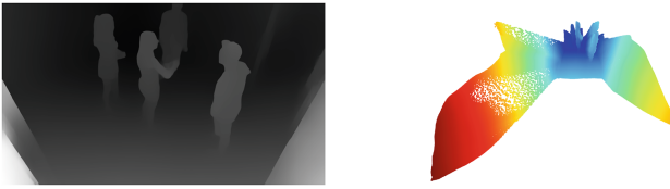
Fig. 3. Conversion of pixel coordinate to 3D Cartesian coordinate; left: estimated depth map, white-to-black color code: close-to-far depth distance from the camera; right: 3D reconstructed scene, red-to-blue color code: close-to-far distance from the camera. (Color figure online)
