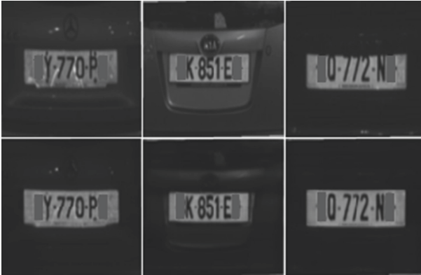
Fig. 3. Results of the plate cleaning method. Top row: Faulty samples, bottom row: their cleaned counterparts. Note how in the leftmost example, the cGAN did not only fix the contrast but also removed the specs above the Y and P character.
