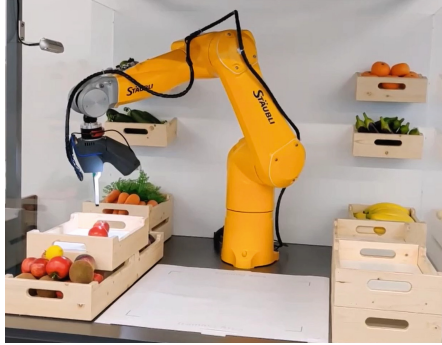
Fig. 1. Showcase of a robot sorting different types of fruits used to demonstrate fast retraining of new classes. The left basket holds a mix of fruits which are picked up by the robot and transferred to the correct basket on the right. For generation of training images, the new object is placed in the center of the white area (Source: KEBA).
