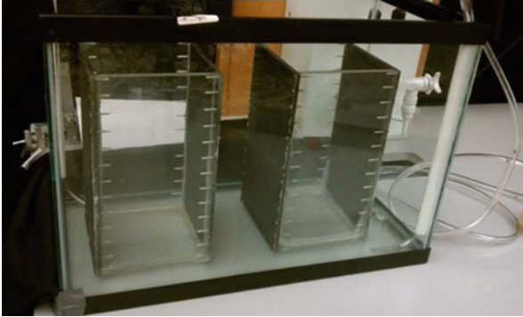
Fig. 3 Setup with two inner experimental tanks and outer tank as a thermal bath which is connected to a recirculating thermally controlled reservoir
