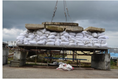
Fig. 8. Stages of loading of research structure
