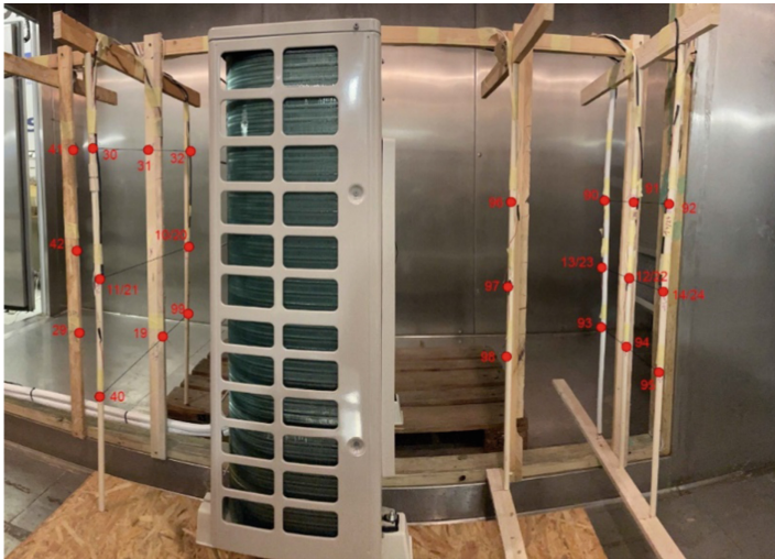
Fig. 6. Sensors around the heat pump
