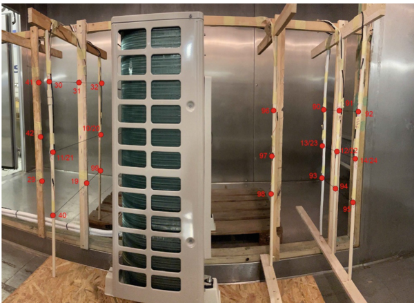
Fig. 1. Location of sensors around the heat pump outdoor unit
