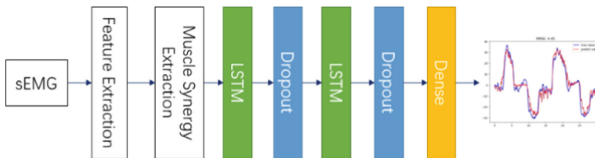
Fig. 2. Force estimation processing flow
