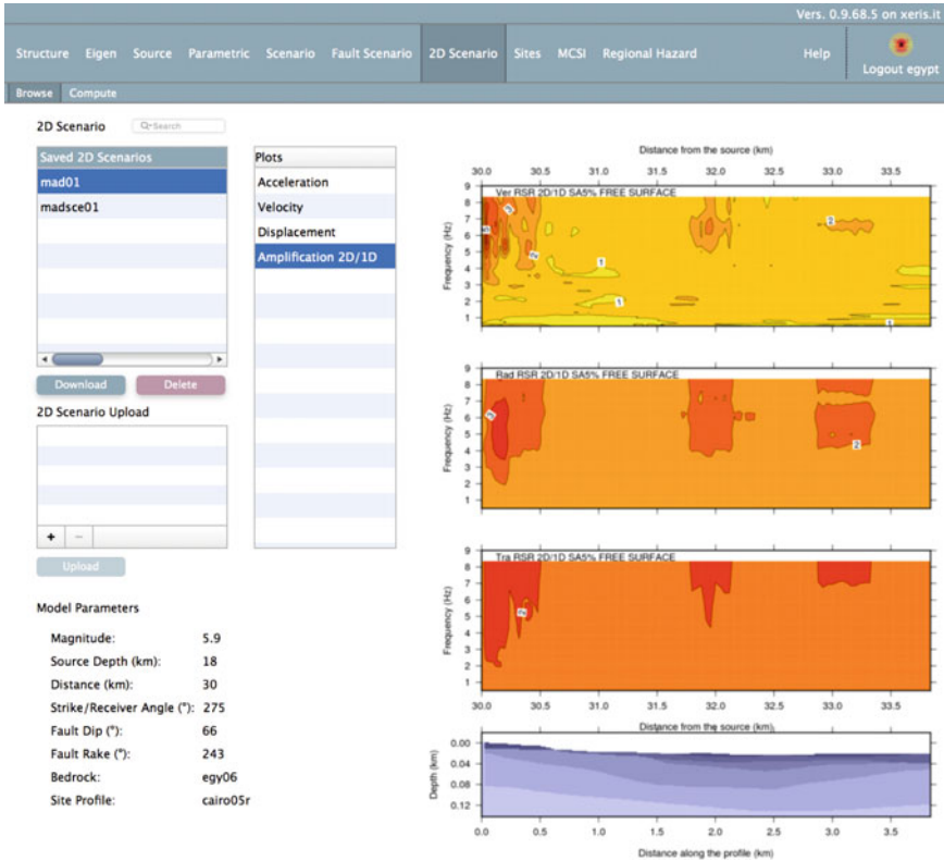
Fig. 9 Amplifications (dark red areas) are shown with respect to a laterally homogeneous bedrock model for the “Madrasa” profile. From top to bottom, the amplifications are shown along the profile for the vertical, radial, and transverse components. The abscissa shows the position along the profile, represented at the bottom, while the ordinates in the upper images refer to the frequencies at which the amplifications eventually occur
