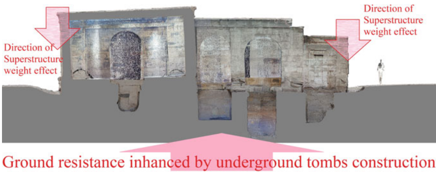
Fig. 16 Cross section through chapels, showing relation between underground tombs and superstructure walls
