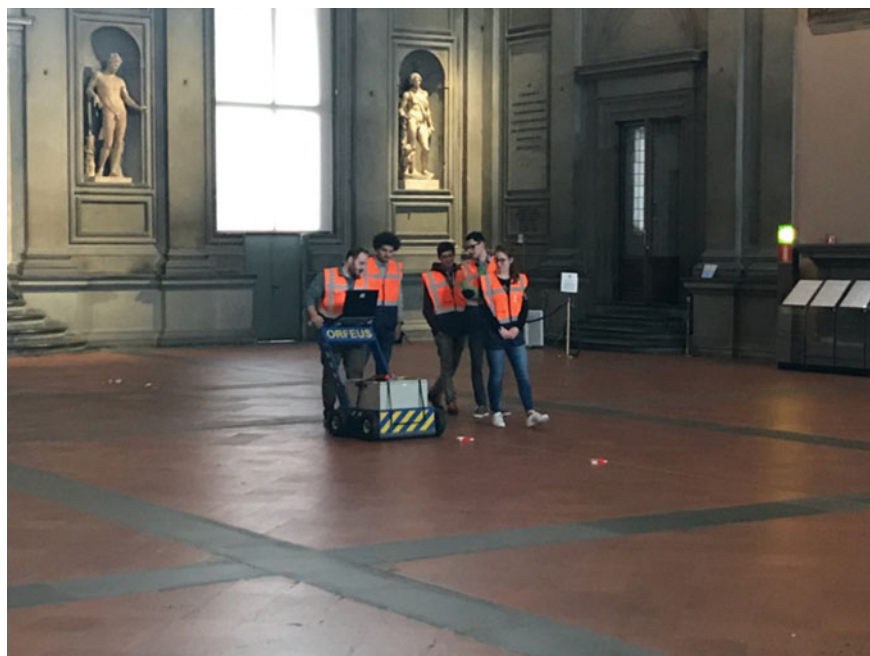
Fig. 6 ORFEUS Ground Penetrating Radar scanning the floor of the Great Hall
