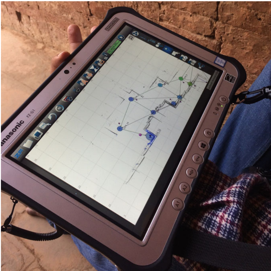
Fig. 5 Real-time registration in the field on tablet using Scout Z+F software (ZF 2019)
