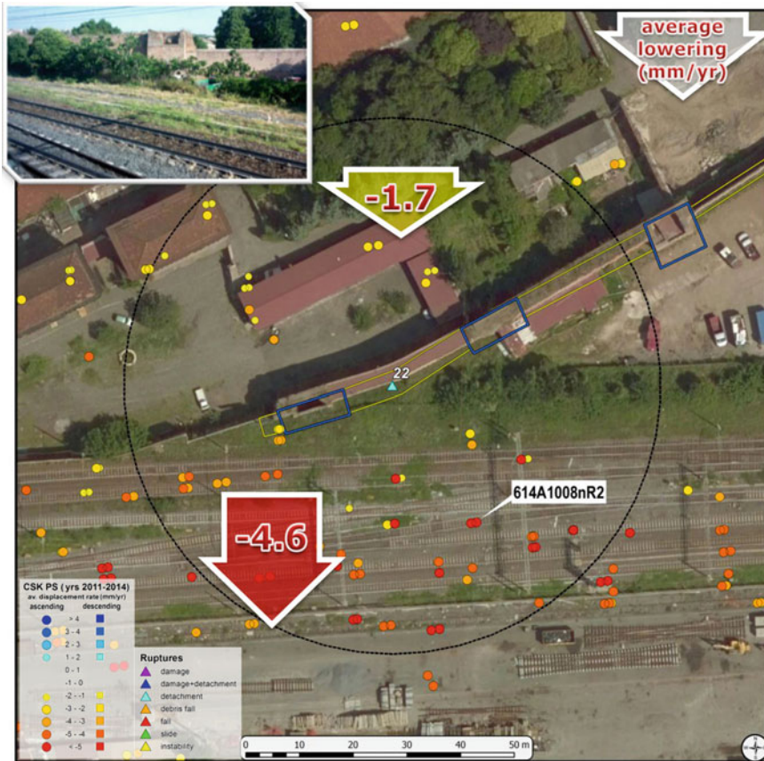
Fig. 10 General subsidence affecting the interaction between walls and railway
