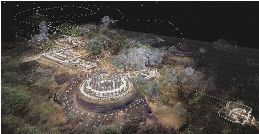
Fig. 3 Screenshot from Reality Capture processing software showing the positions of photos and laser scans needed to capture the site's geometry and texture the monuments. Medirigiriya, Sri Lanka
