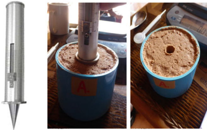
Fig. 13 Yamanaka cone test
