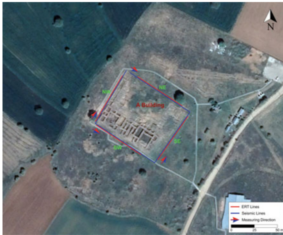
Fig. 25 Plan showing the measuring lines of the ERT, SRT and MASWT studies around the building “A”. The arrows indicate the direction of measurement. NW, NE, SW and SE identify the measuring lines
