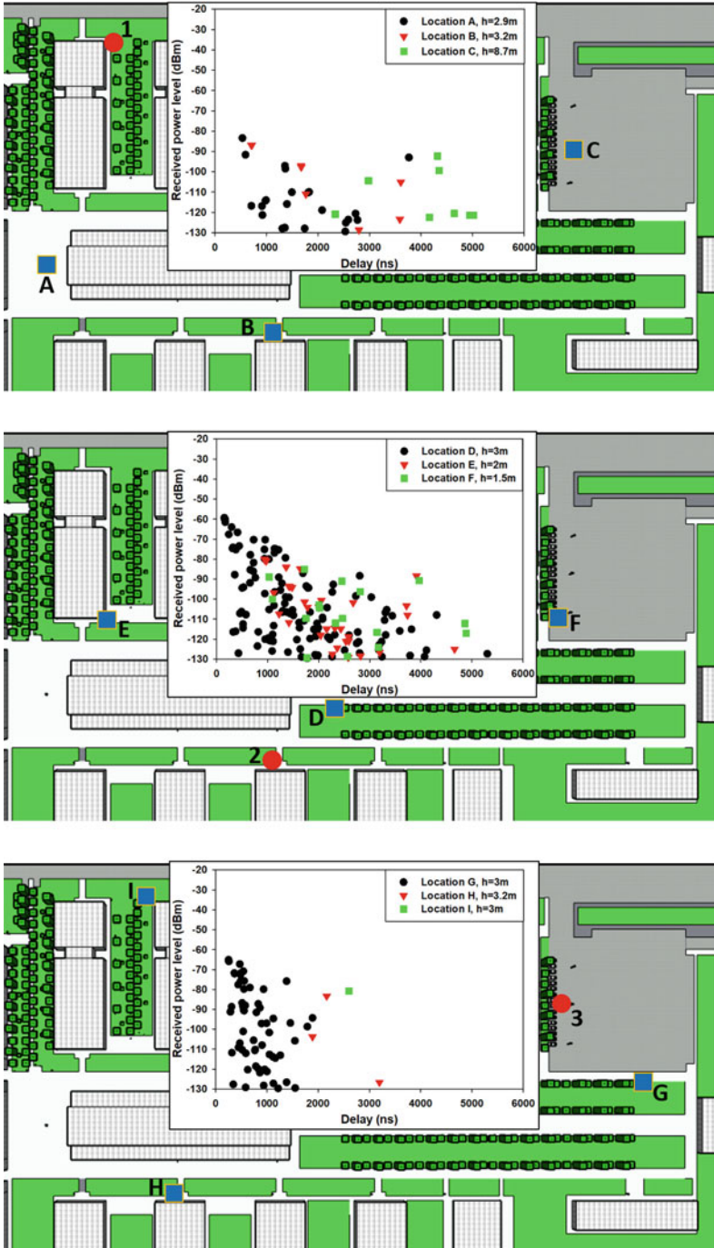
Fig. 8.5 Estimation of power delay profiles for three different transceiver locations, considering frequency of operation of f@868\text{ MHz} . The location for each one of the transceiver locations is given by a red dot within the scenario
