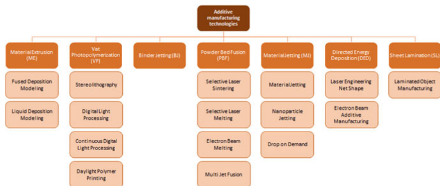
Fig. 2.1 Additive manufacturing technology classification according to the ISO/ASTM 52900-21 standard
