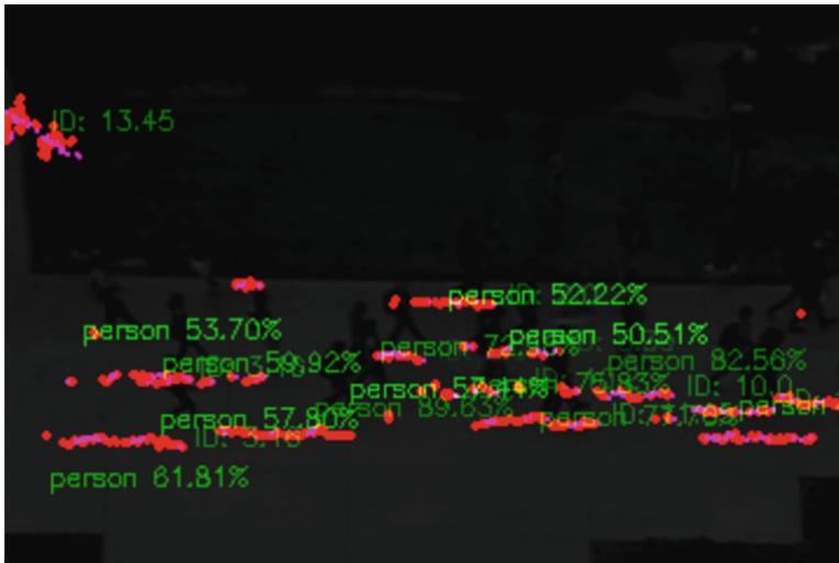
Fig. 6. The first deep learning module consists of the integration of DeepSORT and YOLOv5
