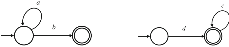
Fig. 1. Two deterministic 1-cycle-free-path-automata: the accepted languages, a^*b (left) and dc^* (right) are d-union-free.
