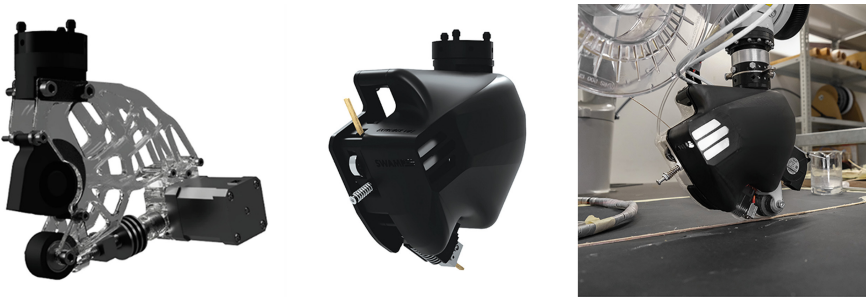
Fig. 5. Example of a 3d printed end effector for extrusion of continuous timber filament, from left to right: internal 3d structure and components, complete model, built extruder.
