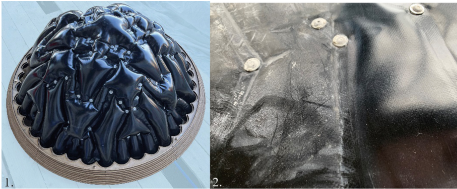
Fig. 12. Inflatible Formwork with support (1). Reusable inflatible Formwork after concrete shell fabrication (2).
