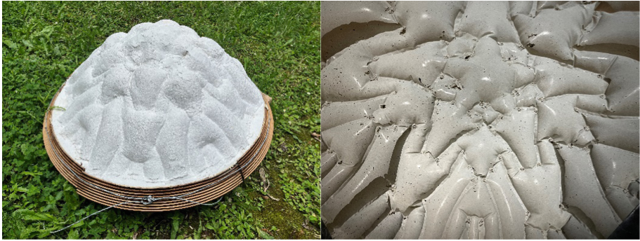
Fig. 13. A concrete shell made with an inflatable formwork.
