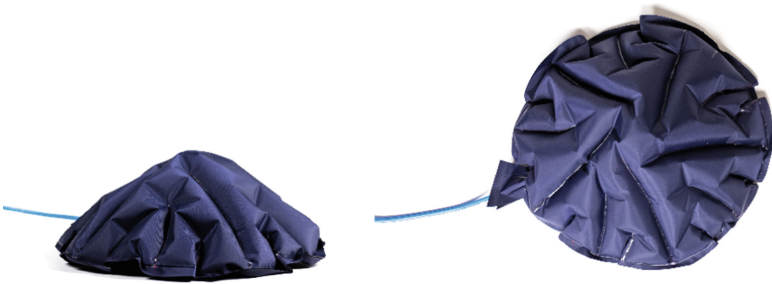
Fig. 3. Manufactured models with 2 sheets of fabric sealed according a 2D pattern.
