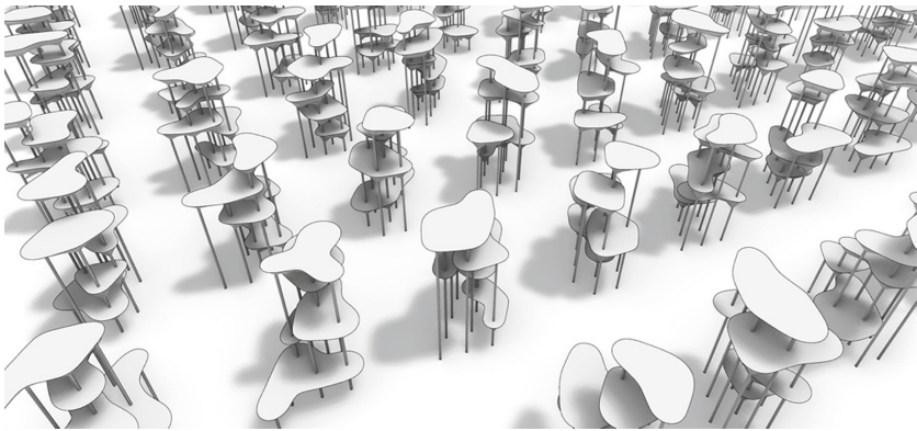
Fig. 12. Different geometries generated from design parameters produced by the AE model, all for the same requested performance attributes.
