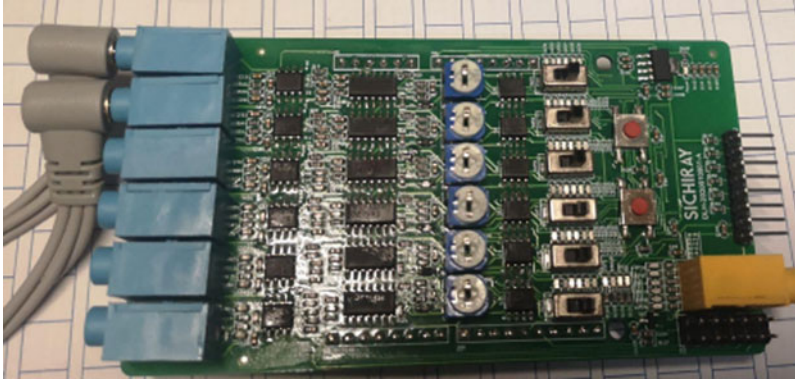
Fig. 2 Six-channel EMG data acquisition device
