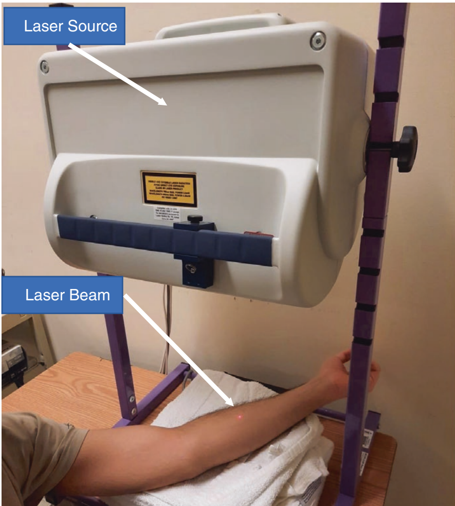
Fig. 16.2 Laser Doppler imaging: A laser beam is emitted from the laser source to sequentially scan a chosen skin area. We employ the scanner to evaluate the area in which hyperemia is produced by the iontophoresed vasoactive substance on the volar surface of the forearm
