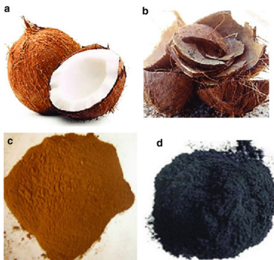
Fig. 1 Coconut (a), nutshell (b), shell powder (c), and charcoal powder (d). Source Photo by the authors
