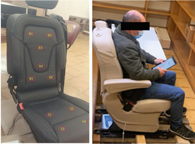
Fig. 1 Seat with the locations where the vibration actuators were installed (on the left), and the final setup (on the right)
