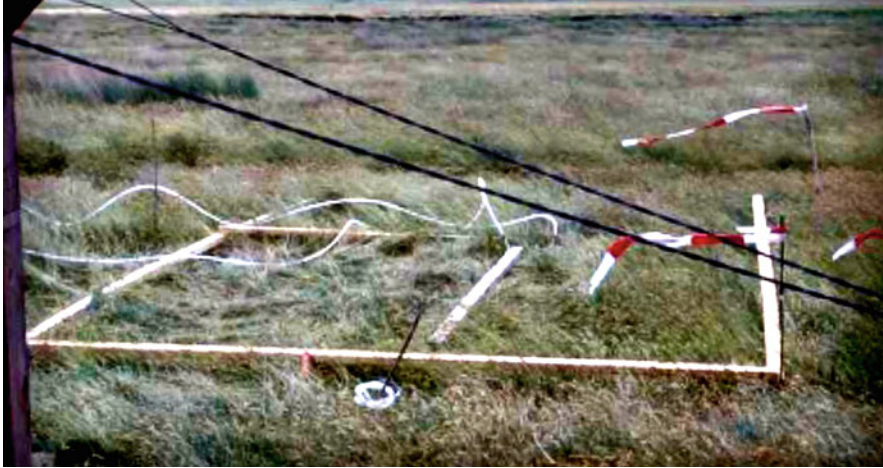
Fig. 16.1 PE tubes laying in the salt marsh of Hedwigenkoog. Experimental and reference sites (each measuring 3 x 3 m)
