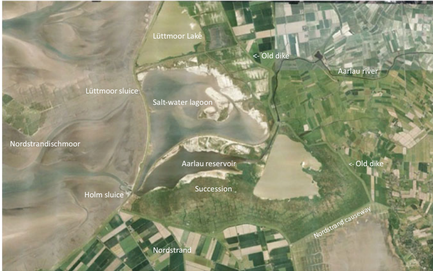
Fig. 22.2 The Beltringharder Koog was finished in 1987 in front of the old sea dike, the isle of Nordstrand, and its causeway. Satellite photo (Google Earth) from 2008. Salt-water lagoon under tidal influence. Lüttmoor Lake with brackish to fresh water
