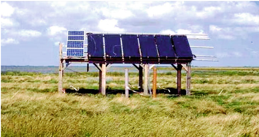
Fig. 16.2 Platform to heat the experimental site. Stage with photovoltaic device for the production of electric power for the control system, logger and pump; solar panel for water heating and station acclimation
