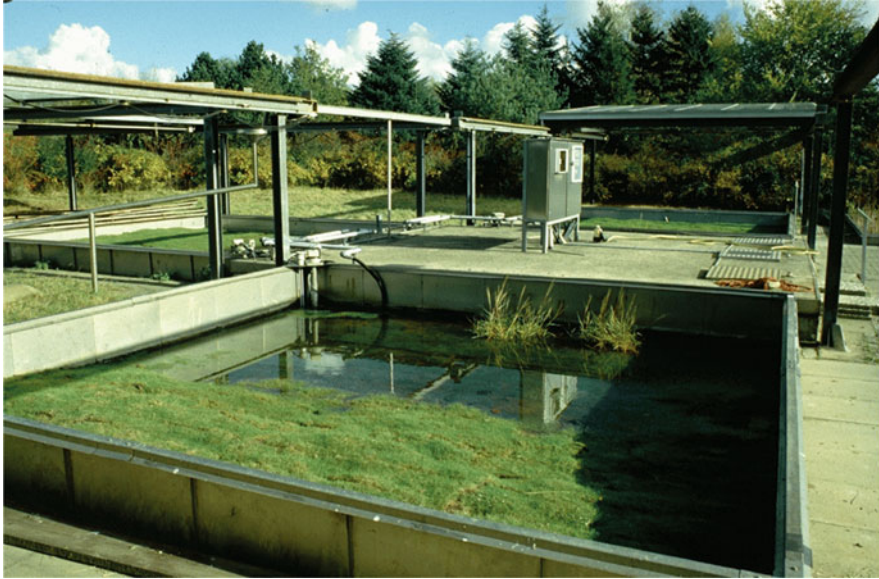
Fig. 20.2 Tide simulation basin half-filled at weekly flood conditions for scenario 1
