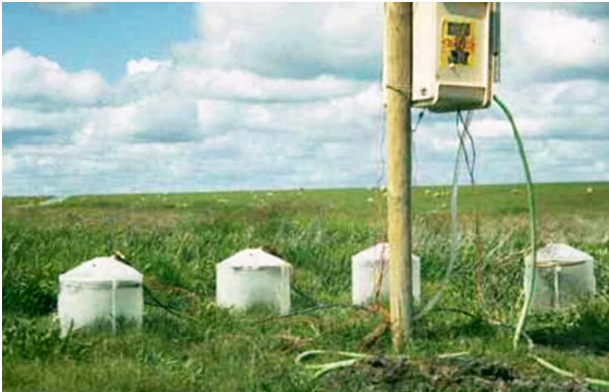
Fig. 16.4 Plexiglas bonnets were used to gather net gas emissions. The mast was fitted with a control device. Inlet tubes for cooling bonnets from above when flooded
