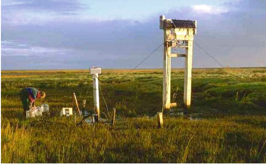
Fig. 16.3 Gauging station in the tidal flat. The station was fitted with a photovoltaic device and Plexiglas bonnets to gather net gas emissions
