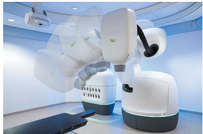
Fig. 10.3 The Cyberknife® (Accuray Inc., Sunnyvale, CA, USA) is a linear accelerator mounted on a six-axis robot that delivers radiation at the target from different positions. The system allows for the detection of patient movement and correction of dose delivery in real time. (Image courtesy of Accuray Incorporated—©2018 Accuray Incorporated. All Rights Reserved)
