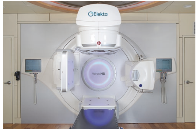
Fig. 10.2 The Versa HD™ (Elekta Inc., Atlanta, GA) is a linear accelerator with a multi-leaf collimating system, which allows for precision shaping of the beam to the treatment area. (Reproduction of photograph courtesy of Elekta, Inc.)
