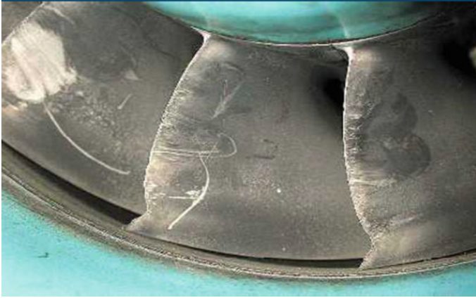
Fig. 3.17 Example of compressor erosion, adapted from Ref. [17]. The image is reproduced under Crown Copyright, with permission from the Defence Science and Technology Laboratory (DSTL). DSTL is an executive agency of the UK Ministry of Defence (MoD)
