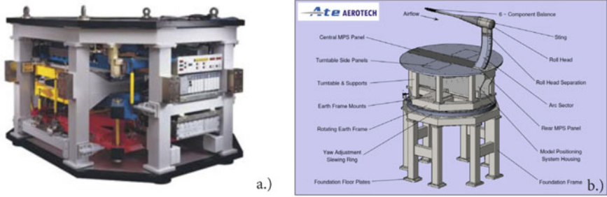
Fig. 2.3 External a and internal b wind tunnel balance systems. The external balance sits entirely underneath or over the working section, and the model is mounted to the balance via struts. (ATE Aerotech, UK)
