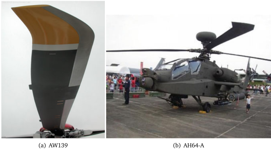
Fig. 1.11 Blade tips of the AW139 and AH64-A helicopters. Credits: a https://b-domke.de/AviationImages/ ; b https://www.airforce-technology.com
