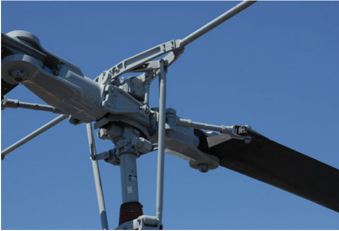
Fig. 1.6 Long pitch-links used on rotor heads. The pitch links will suffer higher loads for high-moment aerofoils used on the rotor. Credits: http://www.grubby-fingers-aircraft-illustration.com/
