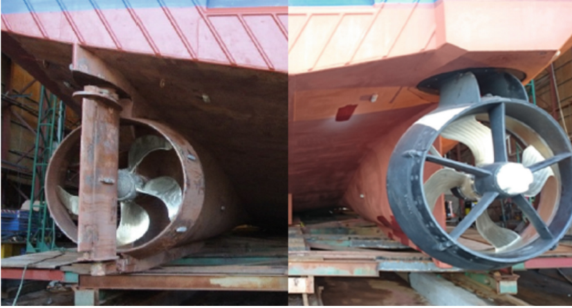
Fig. 2. The propulsion arrangement before and after retrofit.
