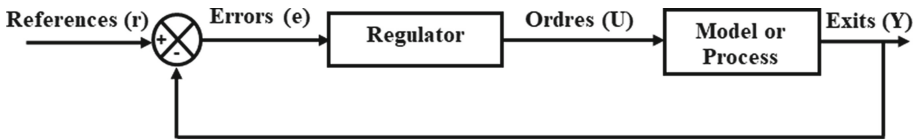
Fig. 2. Synoptic of a regulation law with a feedback loop.
