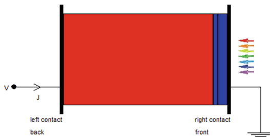
Fig. 1. Solar cell structure of ITO/CdS/GaSe/Mo layer
