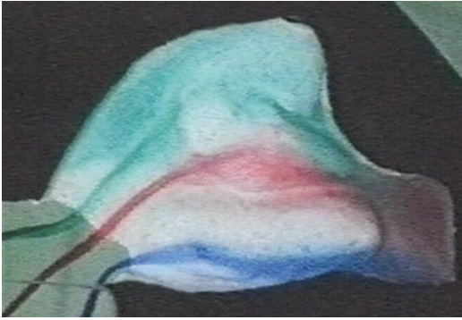
Fig. 20.8 Fluid dynamic experimental representation of the inspiratory airflow in a nose model without a vestibulum. The concavely curved shape of the inner ostium causes a divergence of the flow paths in the cavum
