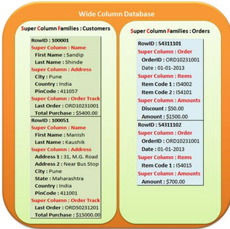
Fig. 7 NoSQL Wide Column Database (“Graph Databases: NOSQL and Neo4j,” infoQ, [Online]. Available: http://www.infoq.com/articles/graphnosql-neo4j [Accessed 26 March 2018].)
