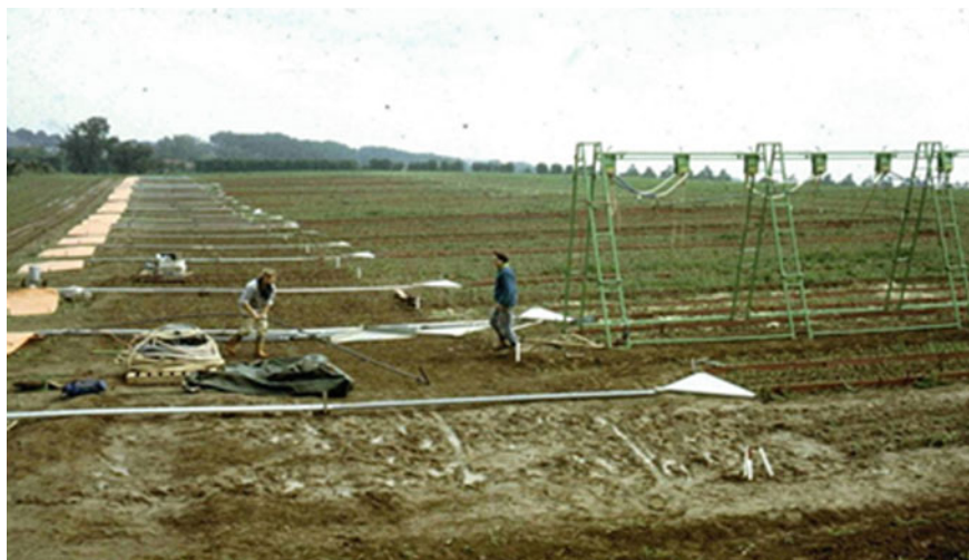
Fig. 5 Rainfall simulator, Experimental Farm Wijnandsrade, South-Limburg, The Netherlands after [50]
