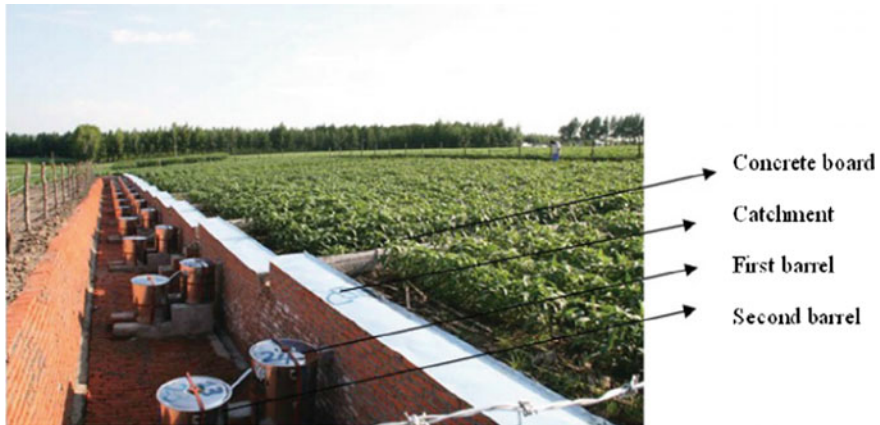
Fig. 4 Collecting sediments from runoff plots. Hailun field experimental station, Heilongjiang, China after [30]
