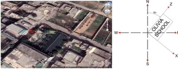
Fig. 8 Angle of building with north axis and components
