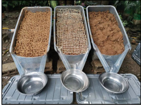
Fig. 7 Experimental Test Beds with coconet (left) with PALFNet (middle) and bare soil (right)
