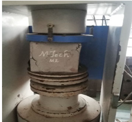
Fig. 6 Crack propagation pattern of cube sample at failure
