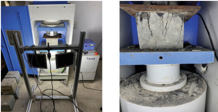
Fig. 1 Data acquisition setup and sample concrete cube under compression load
