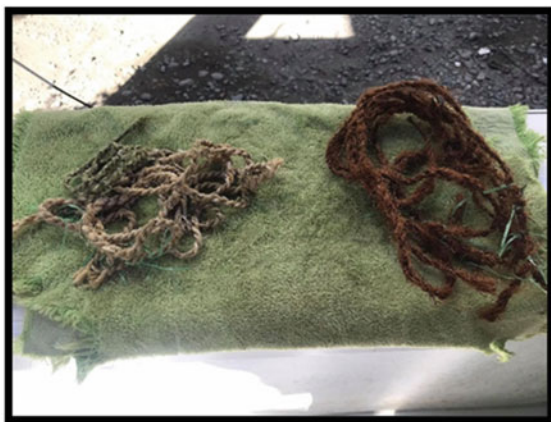
Fig. 6 PALF ropes and coco twines pat-dried with a clean cloth
