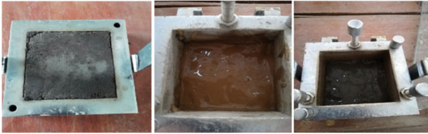
(a) Without drilling fluid (b) With 8% bentonite slurry (c) With 0.05% polymer slurry
