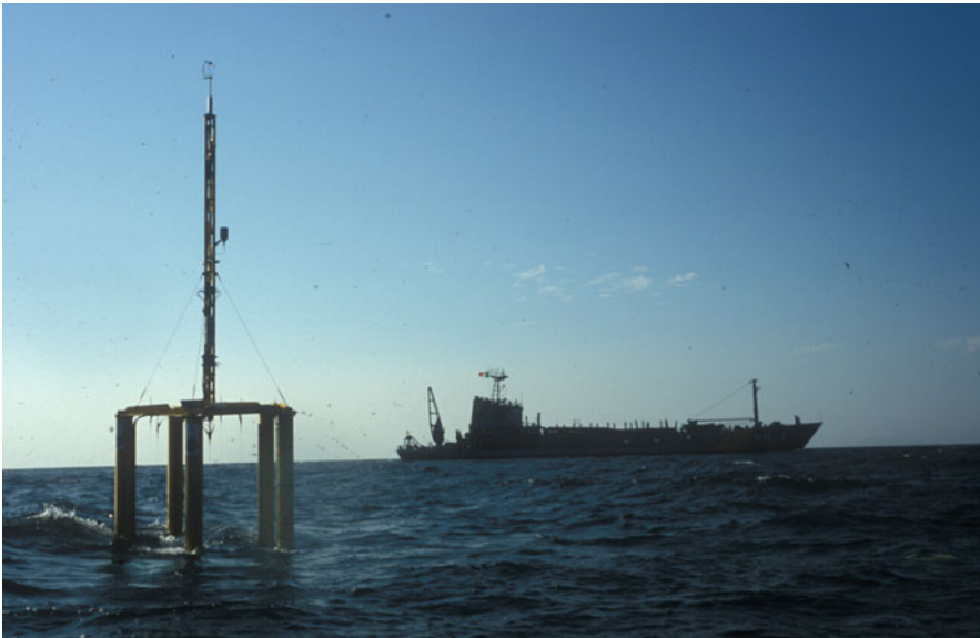
Fig. 1 Air-sea interaction spar (ASIS) buoy deployed in 2005 in the Gulf of Tehuantepec, Mexico, during the INTOA Experiment [36], with the support of the DR06 Bahía Tepoca vessel from the Mexican Navy (Secretaría de Marina-Armada de México), as seen in the background (Photo: S. Ramos)
