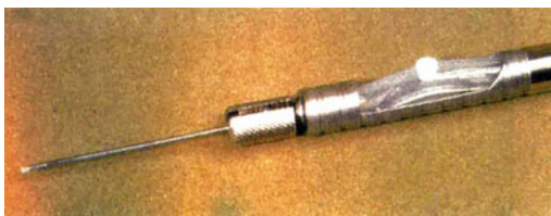
Fig. 1.5 Back-flush needle with silicone tip
