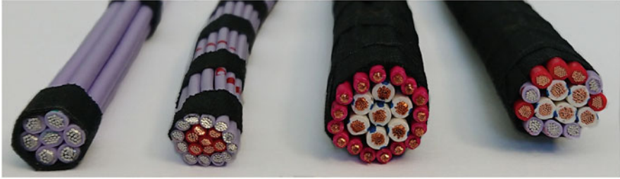
Fig. 1 Examples of different types of bundles with different taping patterns: partly, half and fully, from left to right. The single cables are arranged in layers or randomly (right)
